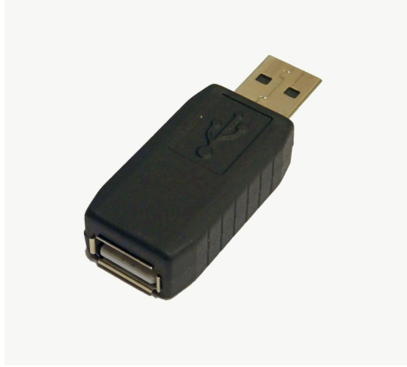
Figure 2.2: Example of an Inline Hardware Keylogger [6]
